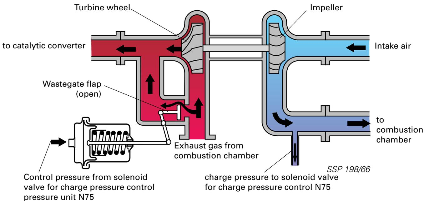
If there is no flow, N75 is closed and the charge pressure acts directly on the pressure unit. The waste gate opens even if the charge pressure is low.
