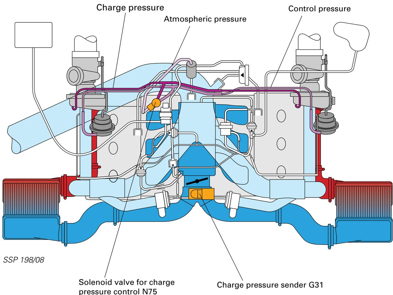
The solenoid valve for charge pressure control N75 changes the opening time to atmospheric pressure according to the signals it receives from the engine control unit (duty cycle).
