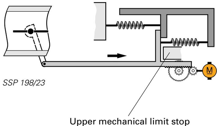
To enable the exact angular position of the throttle valve to be identified, angle senders for throttle valve drive G187 and G188 must be learnt .
