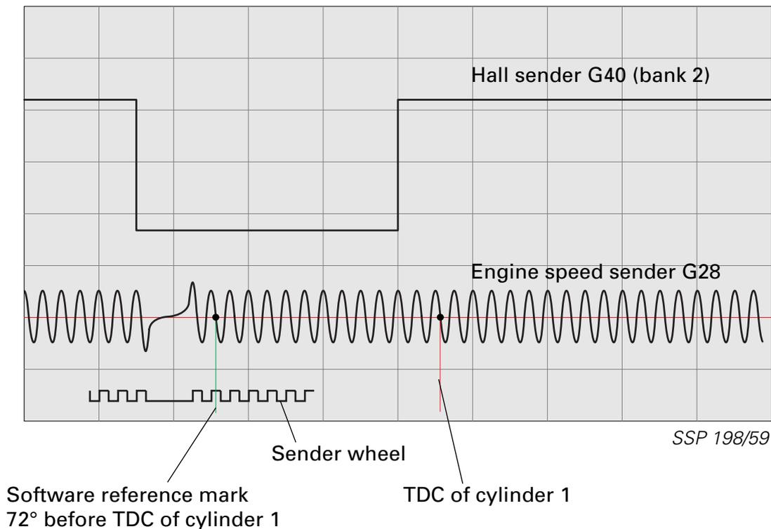
**Diagram of signal of engine speed sender and the two Hall senders**
