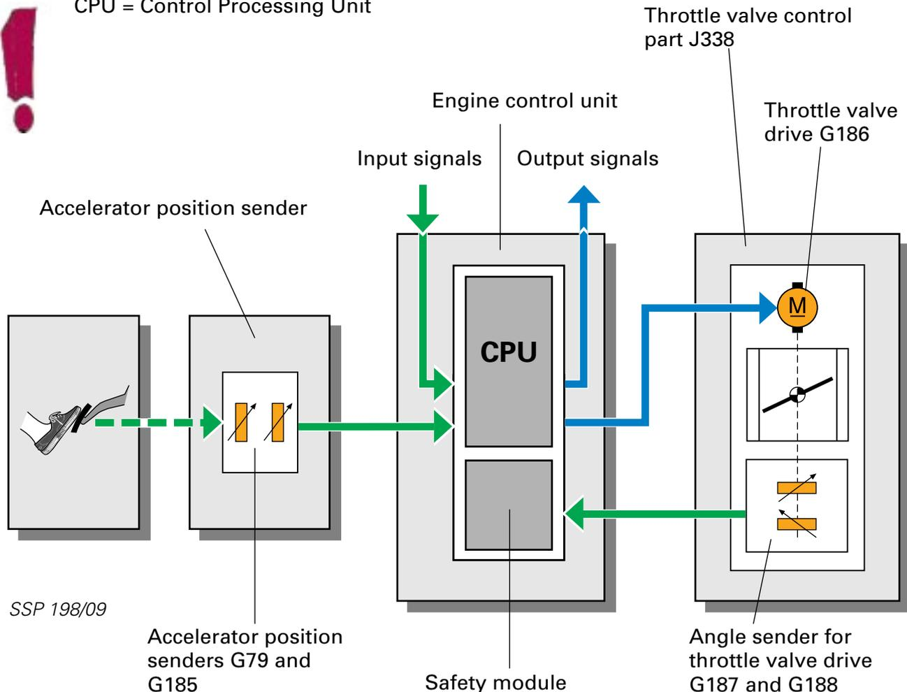
The electronic accelerator controls the engine output electronically and, over and above intake-air control, offers the advantage that functions such as idling speed control, cruise control or engine governing can be executed easily and comfortably.
