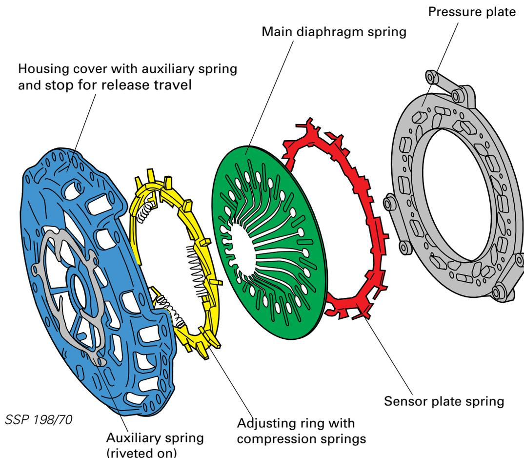
Unlike conventional pressure plates, the main diaphragm spring mounting of the SAC clutch is non-rigid.
