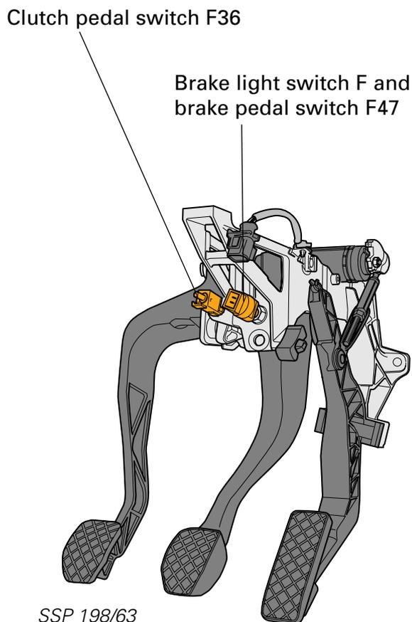
The information “brake operated” is required for the following functions:
